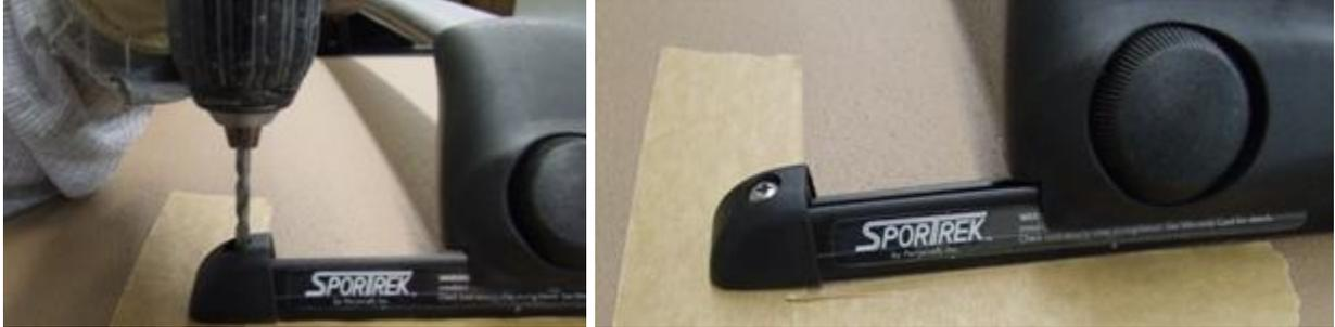
5. After all the holes are drilled, remove the roof rack from the hardtop. (**Reassemble the same as it was removed as the holes in the Side Rails may be in different locations**) Eliminate all debris and clean all of the exterior holes on the hardtop and the bottom of the Side Rails with alcohol to ensure a leak free fit. Install the (10) Foam Washers onto the Side Rails and the End Caps.
