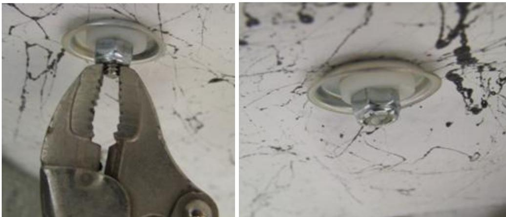
10. Install the Snap-On Covers (10) to all of the Retainer Washers. Install Stanchions and Crossbars to desired positions. **(Caution be sure to tighten the Adjustment Knobs before traveling)**
