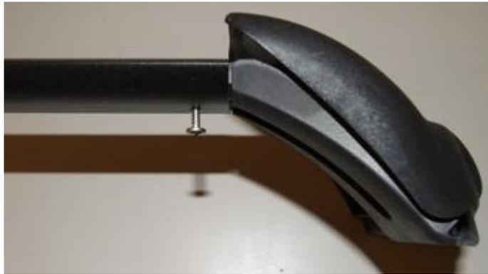
2. Assemble the roof rack on the hardtop and leave the Stanchion Assemblies loose to allow for alignment.
