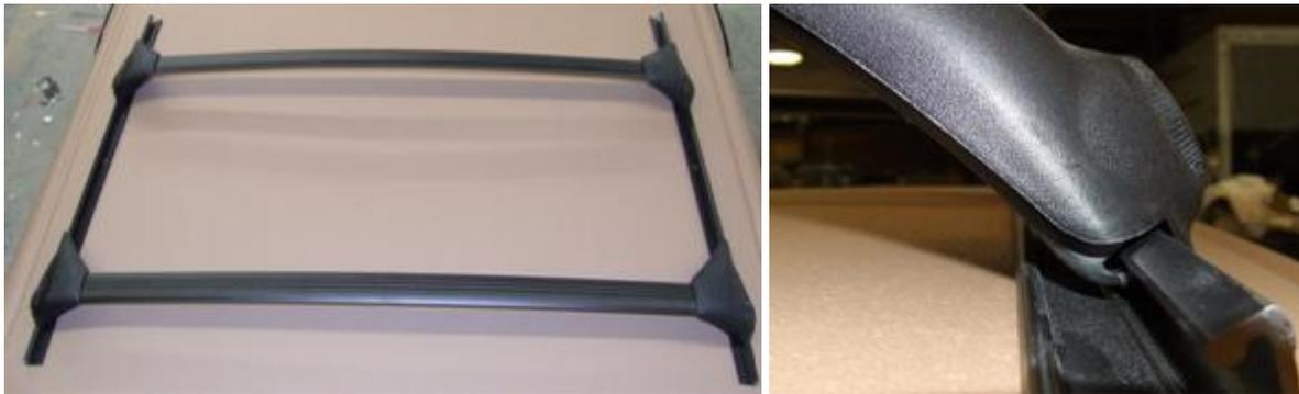
3. Measure @ 2 1/2" inches from the center of the back end of the rain channel to the outer edge of the Side Rail on both sides. Then measure the rail @ 3 1/2 inches from the center of the front end of the rain channel to the outer edge of the Side Rail on both sides. (**This will take several checks to assure equal alignment as movement can/will occur**) Once correct measurement is achieved, place pieces of tape on the hardtop around the Side Rails to indicate if any movement has occurred.
