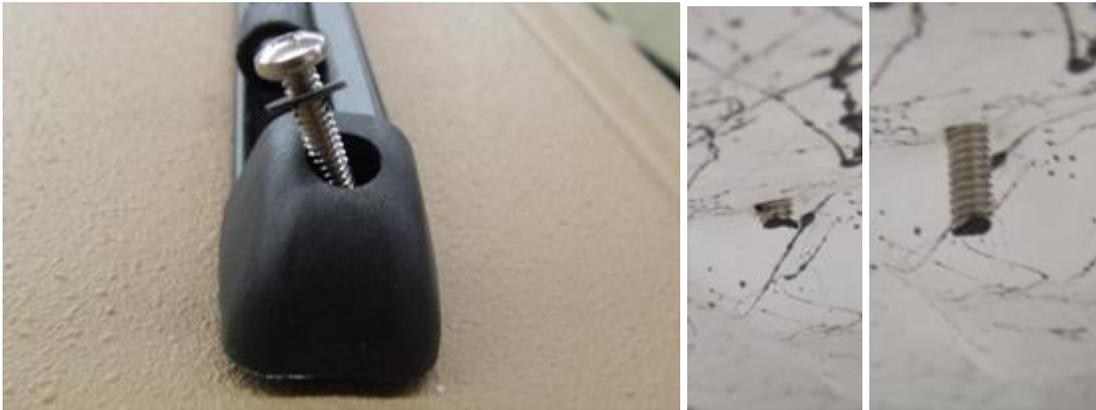
8. Install the Retainer Washer, Nylon Washer and the Nylok Nut to the bottom of the screws. Tighten using a 3/8" nut driver or socket and a drill or screw driver. Be careful not to over tighten.
