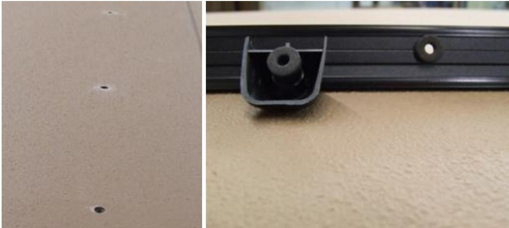
6. Place the Side Rails back on the hardtop and install the Tie Down Loops (4) on each end of the Side Rails.
